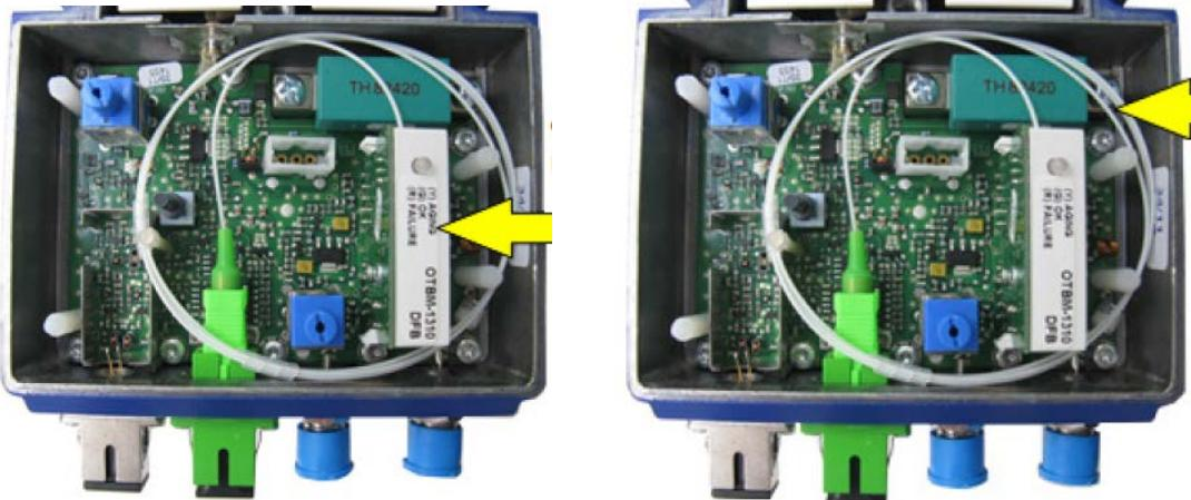
3. Insert the **T0 LR xx xx** and connect to the output connector
