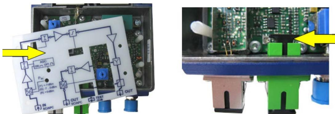
1. Remove the cover that protects the PCB
