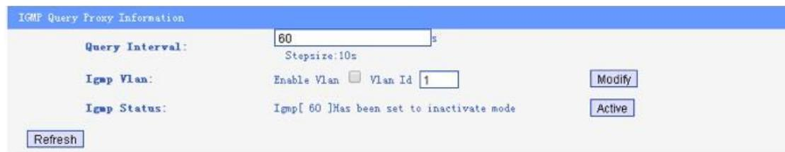
The screenshot shows the 'IGMP Query Proxy Information' configuration page. It includes a 'Query Interval' input field with '60' and 's' next to it, with 'Stepsize: 10s' below it. There is an 'Igmpp Vlan' section with an 'Enable Vlan' checkbox (unchecked) and a 'Vlan Id' input field containing '1'. To the right of this section are 'Modify' and 'Active' buttons. At the bottom left is a 'Refresh' button. The status text reads 'Igmpp[ 60 ]Has been set to inactivate mode'.
