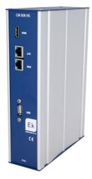
EK HOTEL TV BASIC works as a middleware that allows the aggregation of audio and video services transported in multicast and / or webTV for distribution and reception on IPTV devices (STB IP BASIC).
