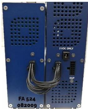
The [FA 55](#) source can also be used to power a single module.
