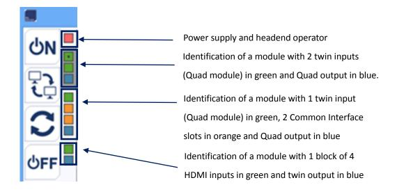
Each module is identified by means of a series of different coloured boxes. Depending on the module, this will be represented by 2, 3 or 4 boxes where the green represents the inputs, the blue the output and the orange the Common Interface slots.
