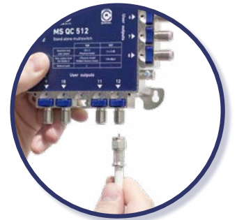
F type connection conversion with AQC-F adapter
