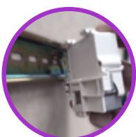
Example of DIN rail mounting
