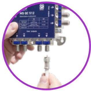
F type connection conversion with AQC-F adapter
