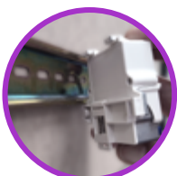
Example of DIN rail mounting
